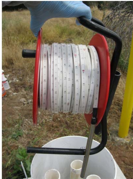
FIGURE 4-3. WELL SOUNDING PROBE AND TAPE
